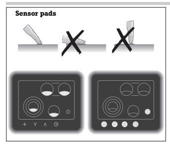
The cooking range is operated by touch control sensors. Touch the required sensor pad in the shaded area as shown in the picture. You only need to touch the pad with your finger, no pressure is required. Every accepted input is confirmed by an audible signal.
